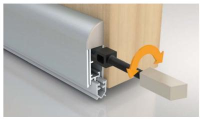
Turn clock-wise: less travel of the seal Turn anti clock-wise: more travel of the seal
